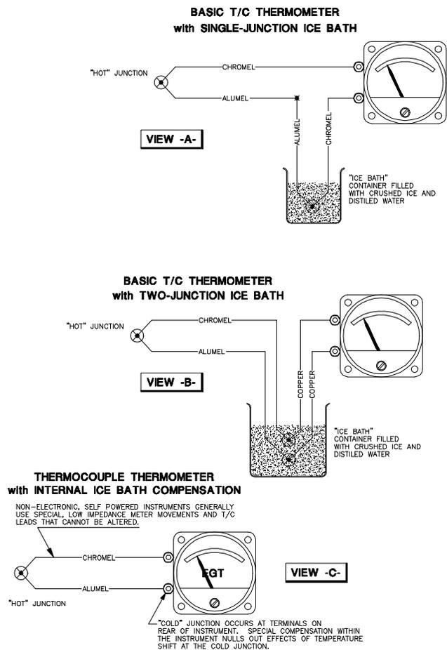
Figure 14-10. Generic T/C Thermometers and Various Cold Junction Techniques.
