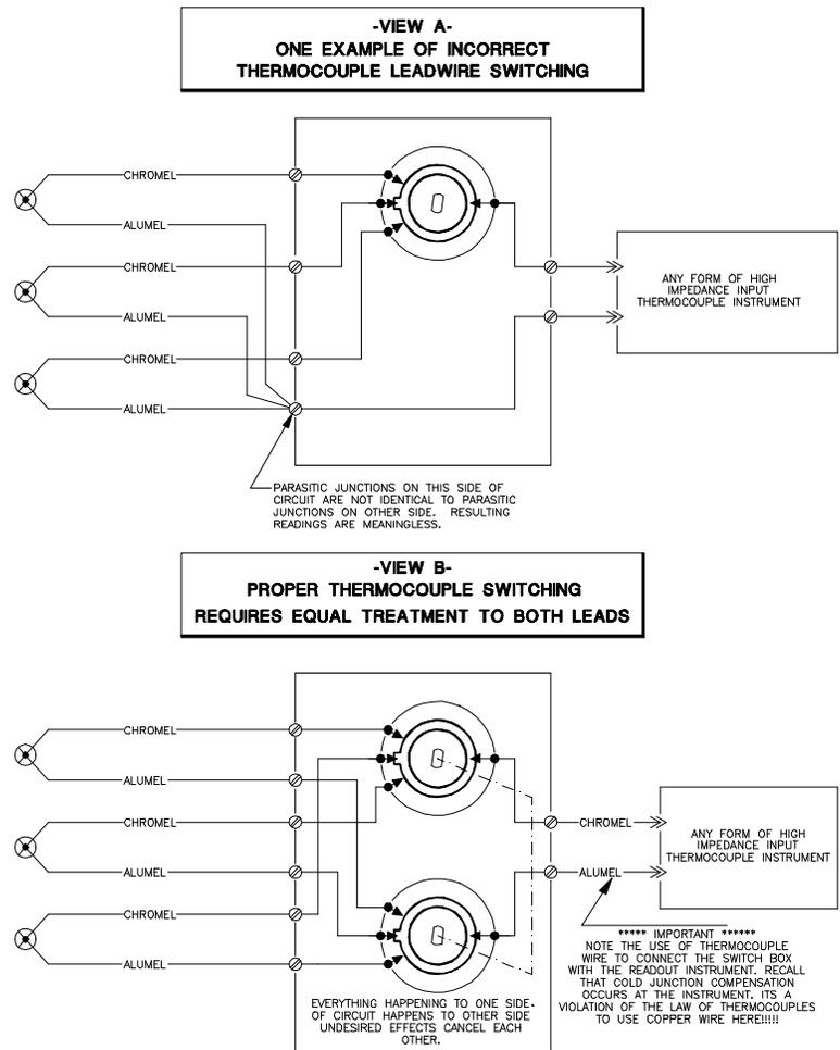
Figure 14-7. Switching Multiple Thermocouples to a Single Instrument.
