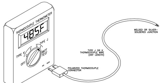
Figure 14-9. Off-the-Shelf Thermocouple Instrument.
