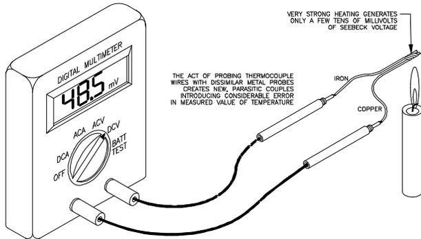
Figure 14-8. Basic Thermocouple.
