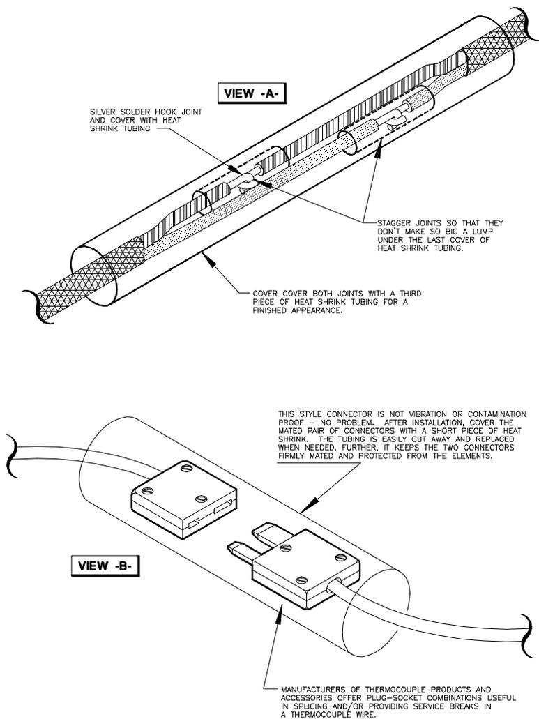
Figure 14-3. Splicing Thermocouples.
