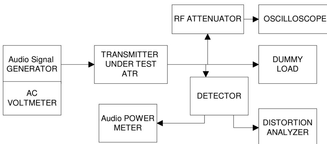
FIGURE 03 – TEST SETUP TRANSMITTER TESTS
