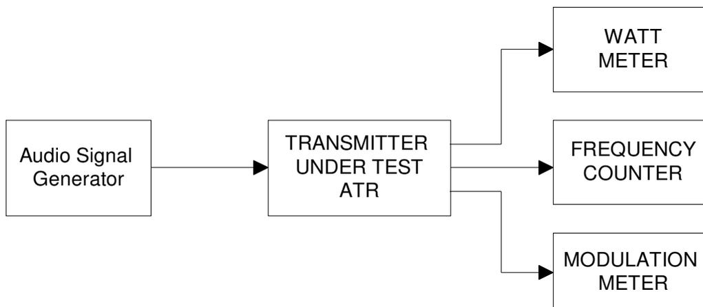
FIGURE 02 – TEST SETUP TRANSMITTER TESTS
