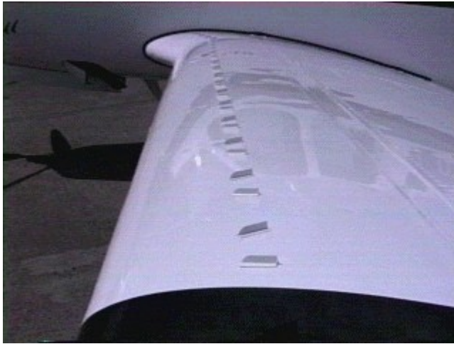
Vortex generator installation on a Beech Bonanza wing.
