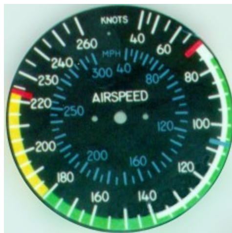
My re-marked airspeed dial. V_{mc} is now below V_s .
