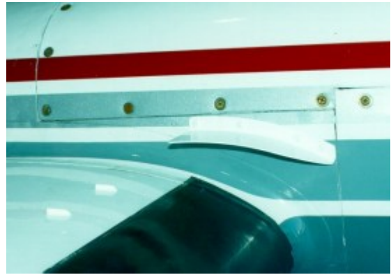
Nacelle strikes bolt on .
