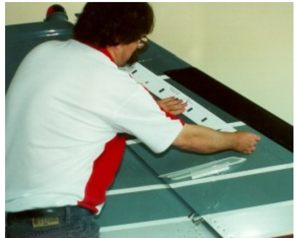
Jay installs vertical stabilizer template along a skin lap. (That giant VG below Jay's right arm is my VOR antenna!) .
