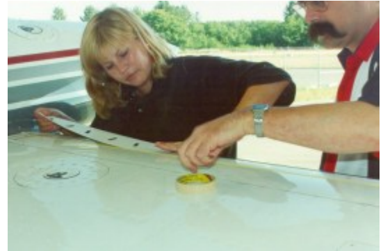
Jean and Jay apply wing template using a taut string.
