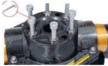
Put all stacked on the propeller shaft (Or on the adaptor spacer corresponding).
