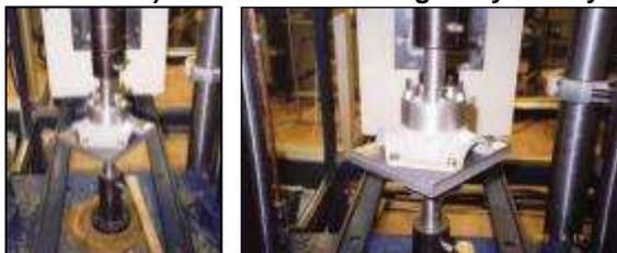
**2<sup>nd</sup> TEST:** Application of a tension along an axis inclined relative to the axis of symmetry of the part
