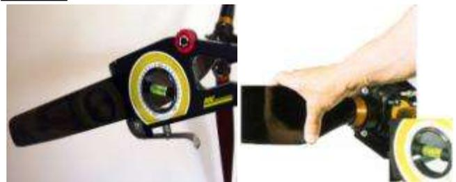
The adjusting of the blade angle is made with a specific tool set. (See 5.3. **Adjusting the blade angle of the propeller**)
