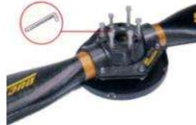
Slightly loosen the screws so that each blade can rotate in its recess without too much effort.
