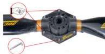
From the front of the hub, set up the 6 short screws for the assembly of the hub.
