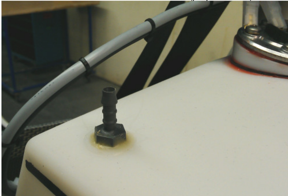
Photo 6: Screw connection for return line (prepared tank)
