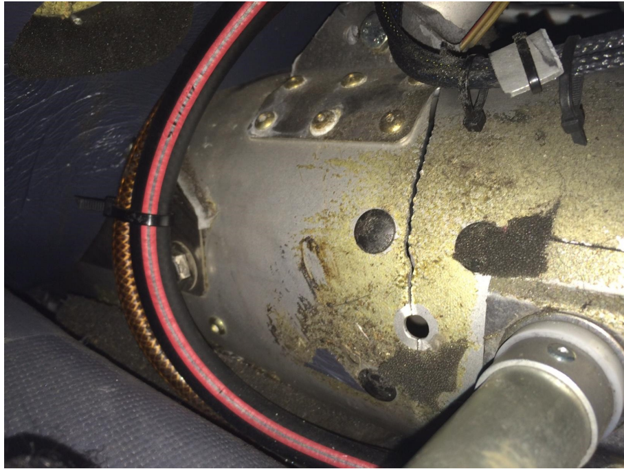
Example of significant crack allowed to propagate on 4500hr aircraft. This crack was hidden by the firewall sound-deadening foam. Ensure that it is removed for inspection.
