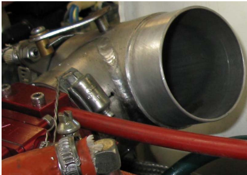
Details of the hot air selector assembly, side view.
