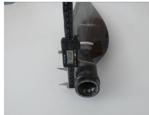
Diameter 45,00 mm (measured by slide calliper)
