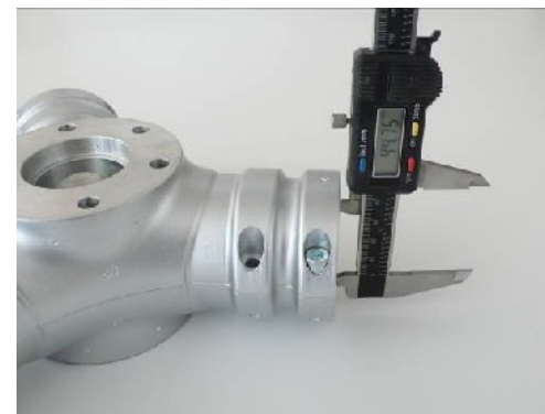
Diameter 44,75 mm (measured by slide calliper)
