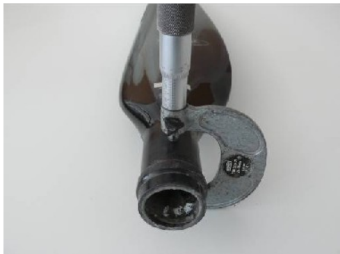
Diameter 45,00 mm (measured by micrometer)
