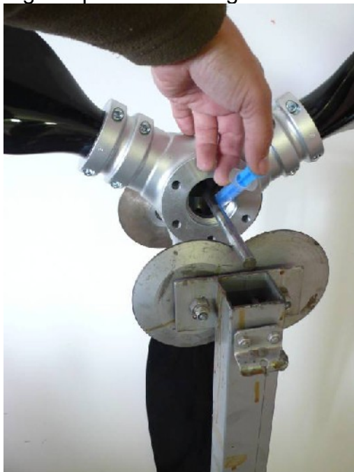
Fig. Propeller balancing
