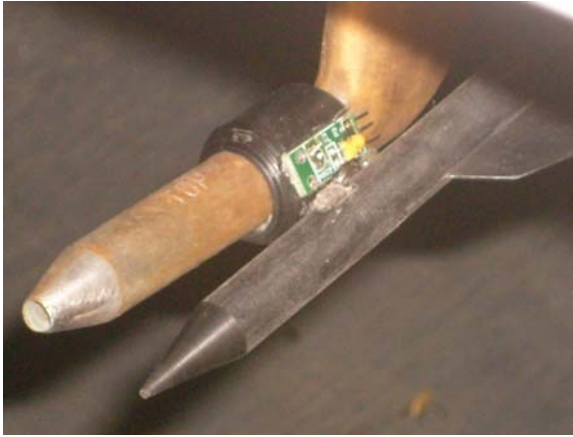
AOA Vane Mounted next to Pitot tube (prototype Connector has been deleted see photo page 2 )
