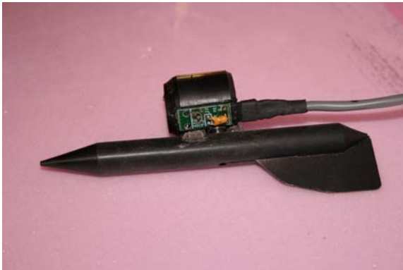
AOA Vane and Mount with Hall Sensor (Cable connector now deleted for production units)
