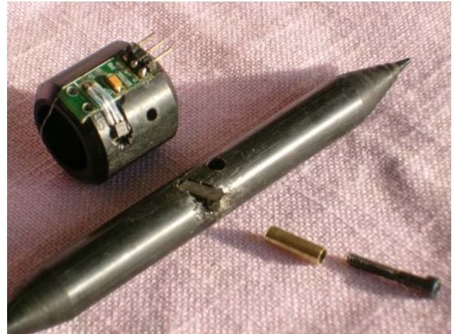
Mount and pivot bearing and vane shaft The bearing surface is between the Delrin Vane and the exterior of the brass sleeve. The brass bearing surface tube is held tightly captive via a 4-40 socket head cap screw. (Small hole holds Hall sensor)
