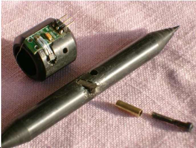
AOA Vane (without fin), magnet and bearing sleeve
