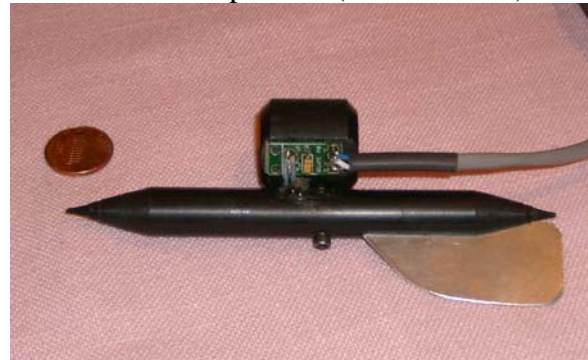
Board with cable and Hall sensor mounted off the side of PC board Note surface mount capacitor (Yellow cube)
