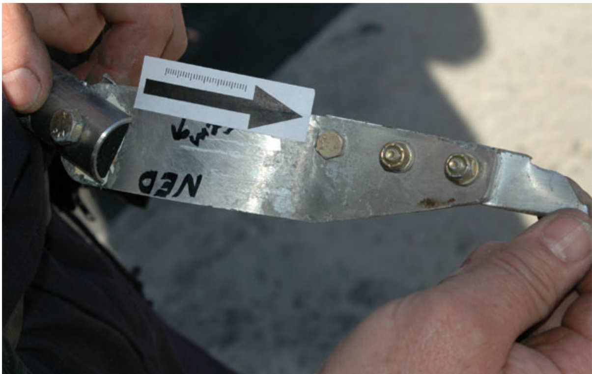
Picture 4: The right-hand wing of the wreck shows a crack at a similar place on the connection plate.
