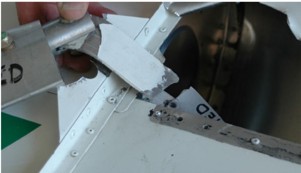
Picture 2: How the connection plate broke near the first bolt at the left-hand wing.
