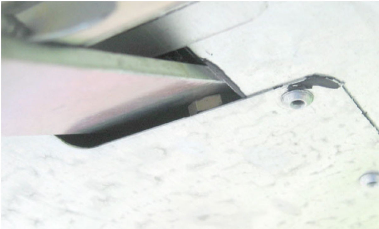
Picture 5: Bright light could improve the quality of the inspection. A suggestion of cutting the plate a few cm to expose the critical location has been proposed.
