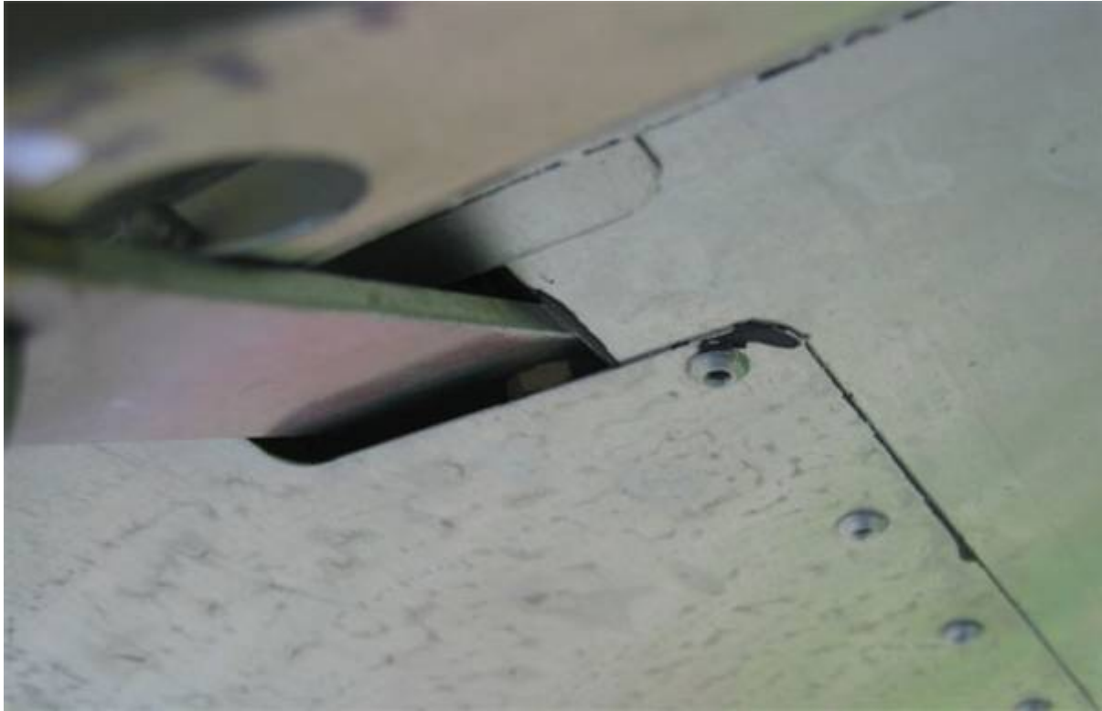
Picture 5: Inspection can be difficult through the narrow slot.
