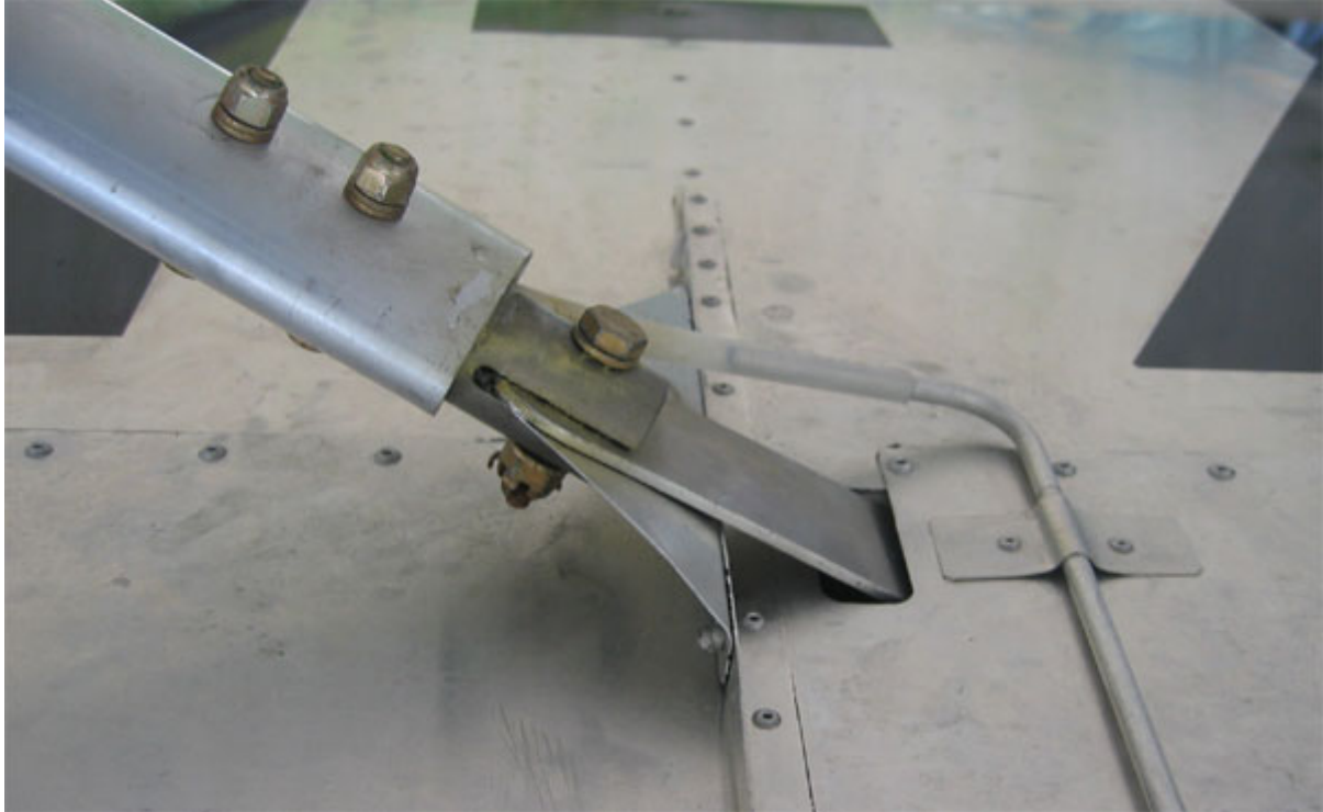
Picture 1: Main wing strut connection plate into the wings main beam. This picture shows an ICP Bingo, which seems to have an identical construction. Picture has been flipped over to resemble picture below.
